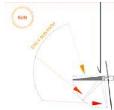
Multifunctional panel: Photovoltaic energy captured during daytime and sun shading
